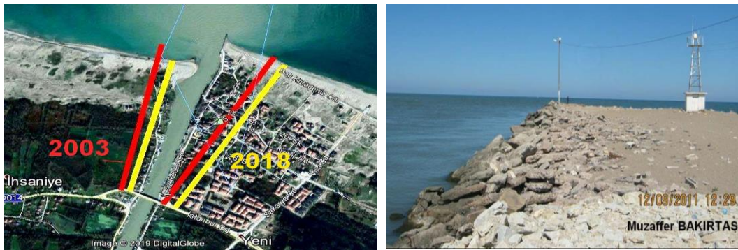
Fig. 5. Coastline change at Google Earth (left) and bank protection in the Sakarya River mouth (right).
