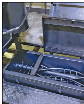
Figure 4. Kneading part of the ProMix D-Helix dough mixer
